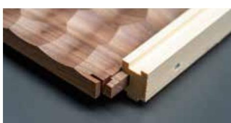
The final finished size is indicated by a saw cut. Minor milling tear-outs along the panel edges are therefore excluded.
